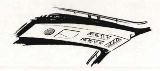
A feature of the M.218/117 is the roof console which incorporates the engine starting controls arranged in sequence, the radio speaker and a cabin floodlight.
