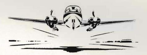
Structure. These aircraft employ a fatigue resistant metal primary structure; the remaining structure is of moulded fibre glass which is a further aid to reliability. A low centre of gravity in conjunction with the wide track undercarriage produces a high degree of ground stability.
