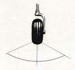
Tricycle Undercarriage. Tricycle undercarriage with steerable nosewheel is standard.
